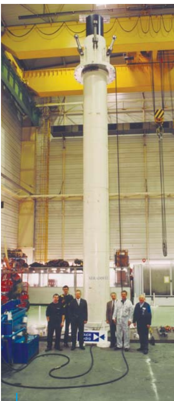
Vertical cast furnace for aluminum platen 1 SA Hydraulic Cylinder rod dia: 790 mm, Stroke 9 700 mm Rod with KERADOUCE® coating
