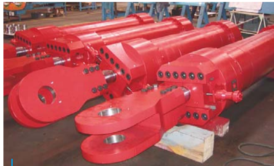
Hydroelectric Dam Baglihar (India) 6 Turbine Cylinders 380 x 240, Stroke 278 mm with locking device
