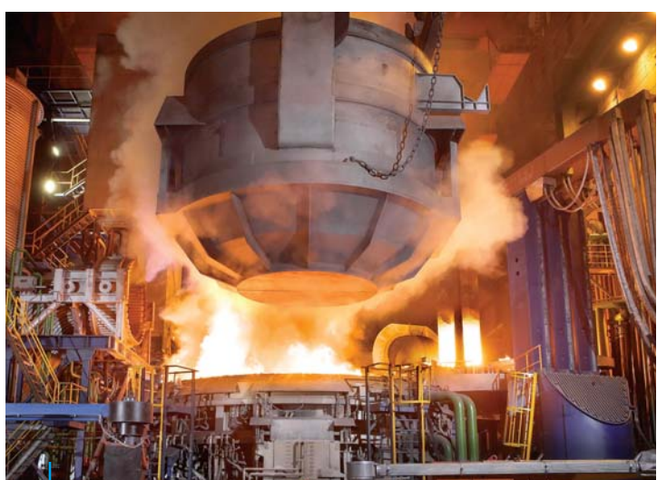
Electric arc furnace
