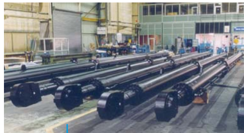
10 Hydraulic Cylinders for radial gates DA 400 x 160, Stroke 17 500 mm with rods in KERADOUCE® coating
