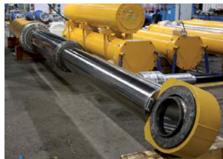
BOP Elevator Telescopic Cylinder 650 x 570, 480 x 380, Stroke 6 100 mm with KERADOUCE® MetalteK™ rod coating
