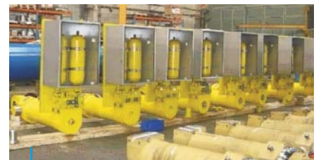
Vertical Lay System Cylinders 32 Hydraulic Cylinders DA 280 x 18, Stroke 550 mm with measuring system
