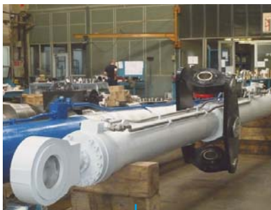
8 Hydraulic Cylinders DA 300 x 130, Stroke 5 600 mm
