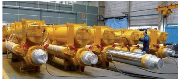
Wireline Riser Tensioner Cylinders DA 540 x 480, Stroke 3 810 mm + HP accumulator dia. 580 mm, Stroke 3 710 mm ; 980 Liters + LP accumulator dia. 304 mm, Stroke 3 450 mm ; 250 Liters
