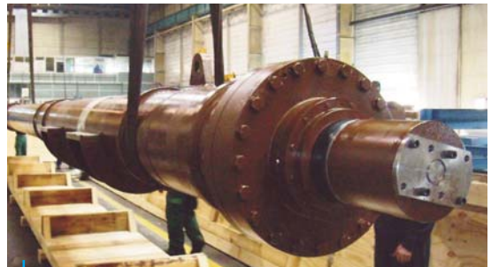
Red River Floodway Expansion Project (Manitoba/Canada) 4 Hydraulic Cylinders 22" x 12", Stroke 43'
