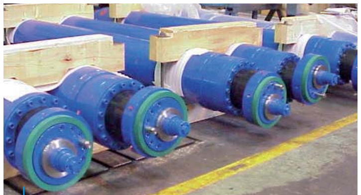
19 Hydraulic Cylinders with rods in KERADOUCE® coating 420 x 340, Stroke 2 700 mm
