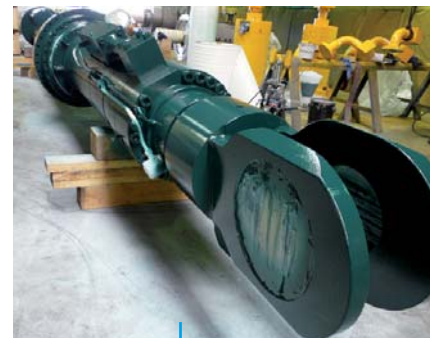
Offshore Dredging Hydraulic Cylinder 1 DA Cylinder 500 x 330, Stroke 8 300 mm
