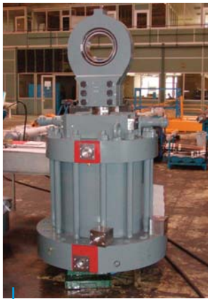
Project Tong Bai (China) 8 Turbine Cylinders 750 x 250, Stroke 440 mm with locking device + 8 Hydraulic Cylinders DA 560 x 200, Stroke 1 913 mm
