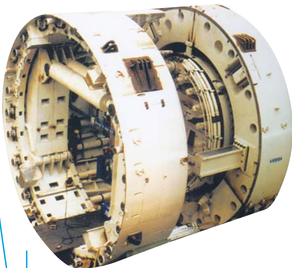
Ping Lin subway telescopic tunnel boring machine (Taiwan) 116 Hydraulic Cylinders in various sizes
