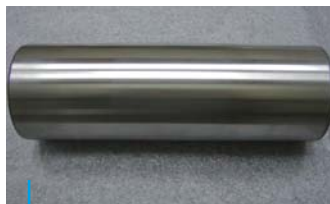
Sample after final grinding and polishing Echantillon après rectification finale
