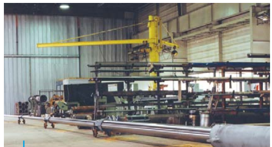
Seaport loading jib cylinder for ships Telescopic Cylinder 4 stages 380 x 280 x 190 x 125 x 100 mm and 21 000 mm stroke.
