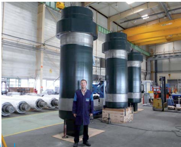
Forging Presses Hydraulics Cylinders SA rod dia. 740, Stroke 2 050 mm
