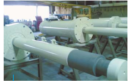
20 Tensioner Cylinders with Transducer
