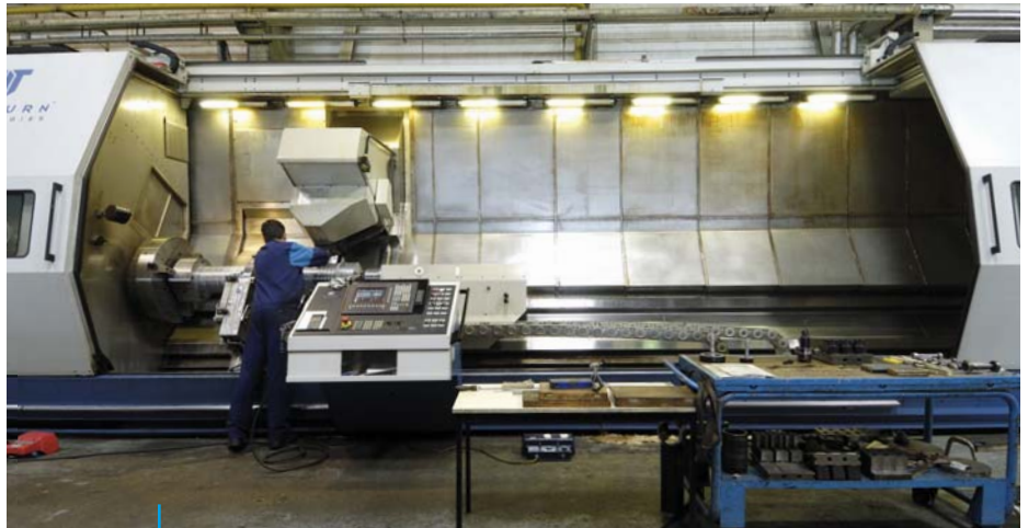
5-AXIS CNC lathe / Tour CNC à 5 axes Swing over top slide: 900 mm / 35 inches Maximal center distance: 6 500 mm / 21 feet
