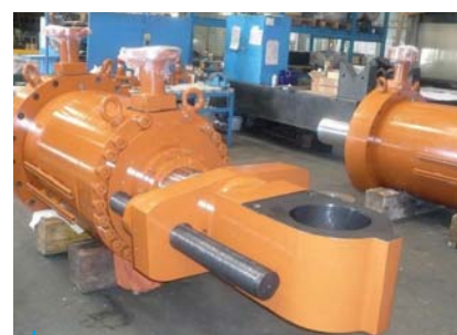
Servomotor Pubugou Dam (China) 6 Servomotors DA 670 x 275, Stroke 549 mm
