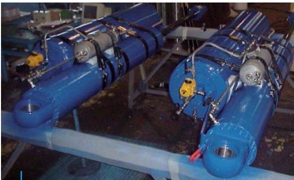
6 Drilling Tensioner Cylinders 222 x 82, Stroke 1 372 mm with high and low pressure accumulators
