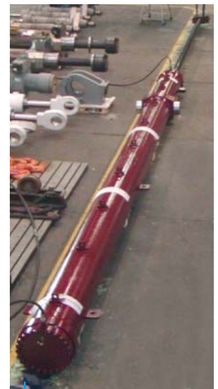
DA Hydraulic Cylinder 500 x 200, Stroke 12 250 mm, Rod in KERADOUCE® coating
