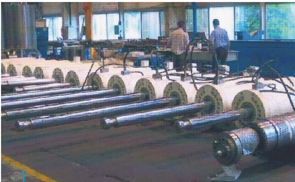
Linear Chain Jack Tensioner Cylinders 32 Cylinders 395 x 171, Stroke 1 612 mm
