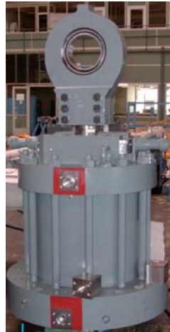
Dam of Tong Bai (China), 8 Turbine Cylinders 750 x 250, Stroke 440 mm with locking device
