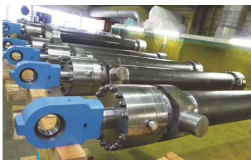
32 holder tilt Hydraulic Cylinders SA 410 x 200, Stroke 3 831 mm
