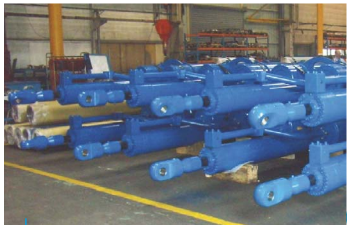
73 Production Riser Tensioners Dia. 260 x 100, Stroke 6 403 mm with 1 low pressure accumulator (20 gal.) + 2 high pressure accumulators (110 gal. each)
