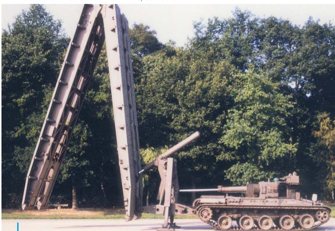
Army mobile bridge / Poseur de pont mobile Hydraulic Cyl. DA 240 x 120, Stroke 2 070 mm Hydraulic Cyl. DA 240 x 120, Stroke 3 070 mm
