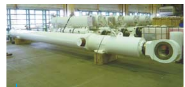
1 lifting Hydraulic Cylinder for retractable turbine DA 510 x 340, Stroke 8 638 mm
