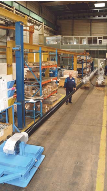
4 Radial Gates Cylinders SA 340 x 190, Stroke 13 100 mm with rods in KERADOUCE® coating
