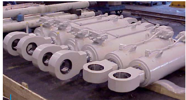
Greece : Rion-Antirion bridge The world's longest cable-stayed bridge with a suspended deck of 2,25 km. 70 Hydraulic Cylinders delivered in different sizes.
