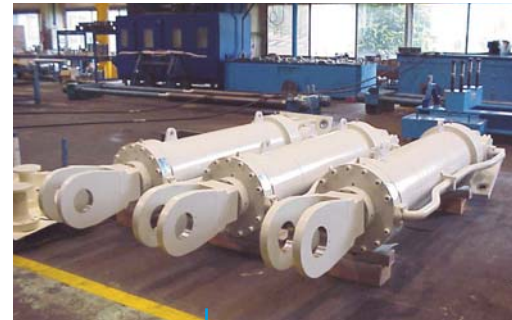
Dam of Yele (China) Rods with KERADOUCE® coating 4 DA Hydraulic Cylinders 440 x 200, Stroke 1 659,71 mm
