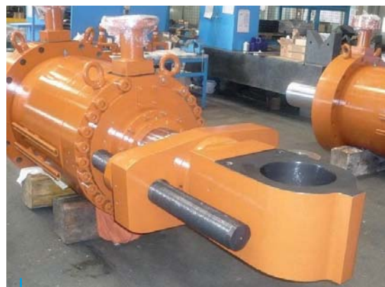
Dam of Pubugou (China) 6 Servomotors 670 x 275, Stroke 549 mm
