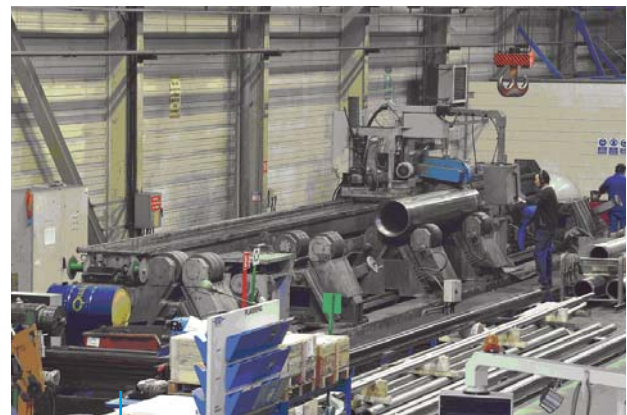
Grinding machine: Diameter: 900 mm / 35 inches Length: 30 000 mm / 98 feet One of the largest grinding machines in Europe !
