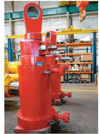
Project Revelstoke (British Columbia/Canada) Servomotors DA 600 x 240, Stroke 580 mm
