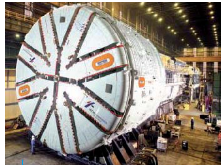
Groene Hart tunnel boring machine dia. 14,8 meters
