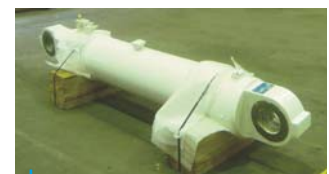
1 counter weight Hyd. Cylinder for retractable turbine DA 300 x 140, Stroke 1 594 mm
