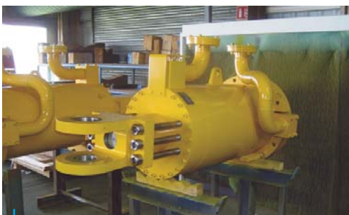
Project Kelsey (Manitoba/Canada) 10 Servomotors 560 x 160, Stroke 686 mm
