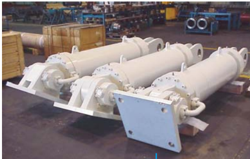
Dam of Yele (China) Rods with KERADOUCE® coating 4 DA Hydraulic Cylinders 440 x 200, Stroke 1 659,71 mm
